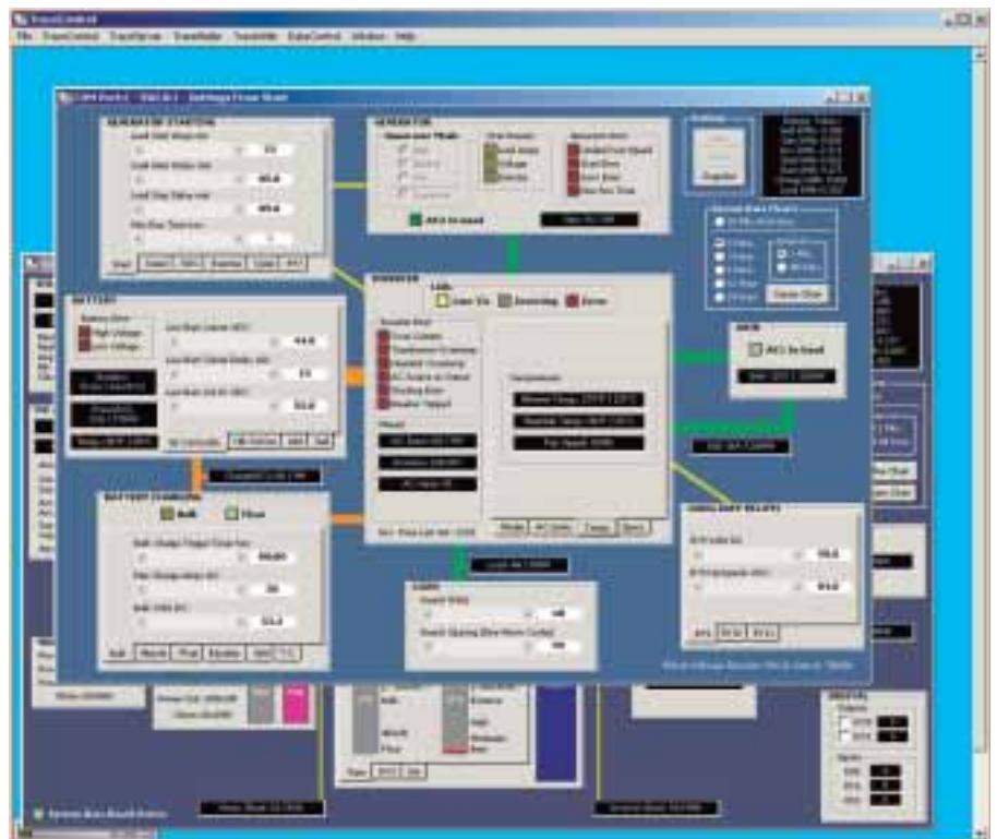
The TraceControl screen allows the user to monitor and tweak the inverter.
