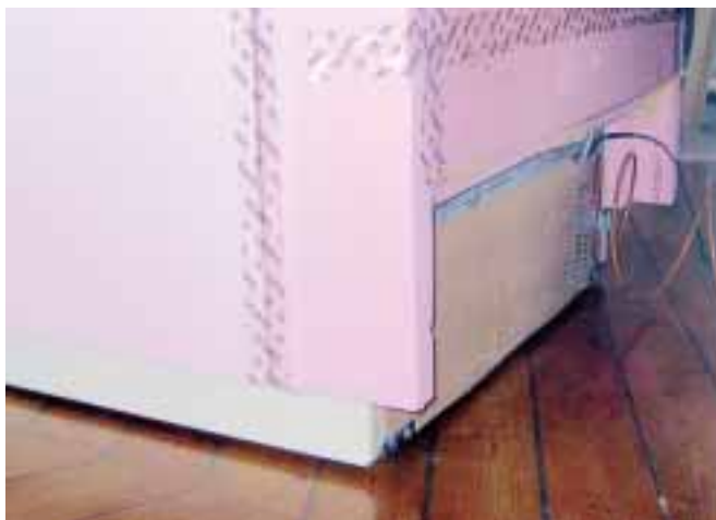
On the lower back, coils and compressor are left uninsulated to dissipate heat.
