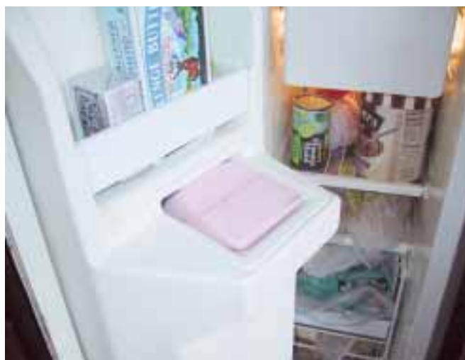
Most of the time, the ice maker is inactive and the opening is plugged with a block of insulating foam.
