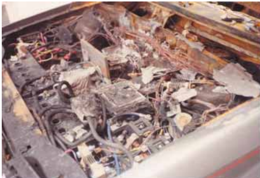
Homebrew electronics with inappropriately rated components can be very costly in the end.
