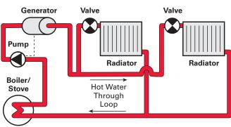
A thermoelectric generator system supplies electricity to a circulation pump installed in a boiler/stove radiator system.
