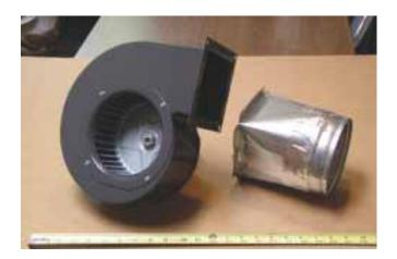
The blower (left) and backdraft damper (right) should be assembled before you crawl into the attic.
