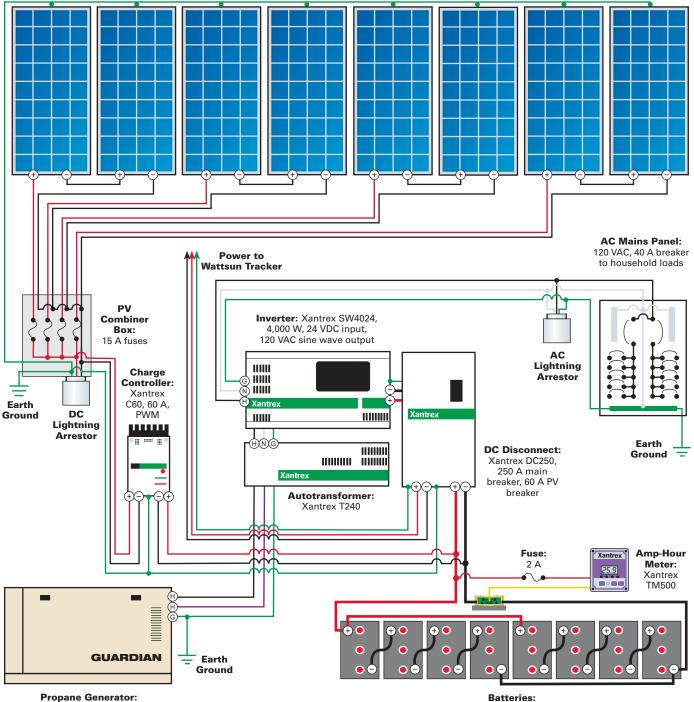
Photovoltaics: Eight Kyocera KC120-1, 120 W each; wired for 960 W total at 24 VDC
