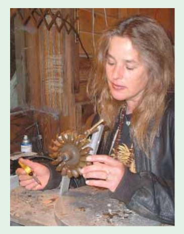
Bliss Kok, Harris' co-worker, carefully assembles the wax plug of a turbine wheel. The wax is cast in plaster, then melted out, after which the plaster mold is filled with bronze. A new wax pattern is used for each wheel.
