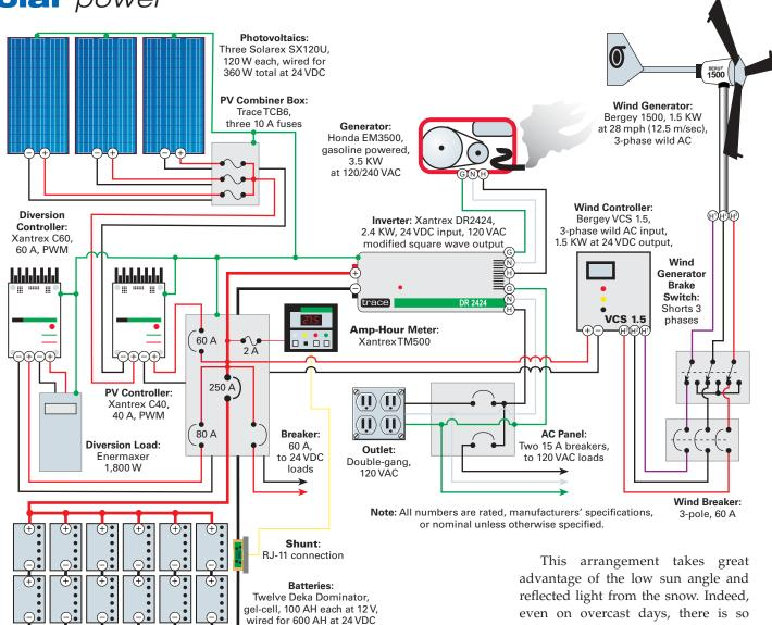
The RE power panel travels to the camp site almost completely assembled. It takes only six connections to make it operational.
