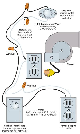
**Note:** All connections should be made in an approved electrical box. Grounds not shown.
