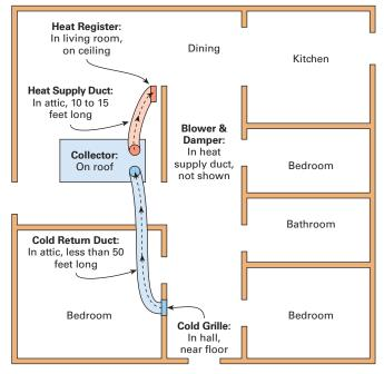
**Note:** Ideal systems have one hot air supply and one cold air return. Multiple ducts can create unpredictable air flow reducing efficiency.
