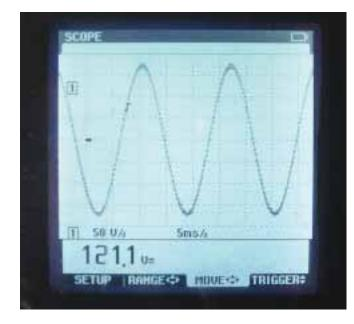
The PureSine 600's waveform displayed on a Fluke 43B.
