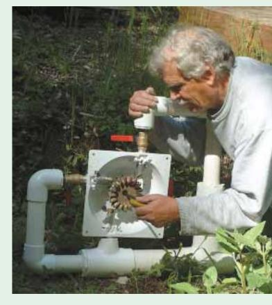
Don Harris holds a turbine on its side to show the four-nozzle layout designed for sites with high flow.
