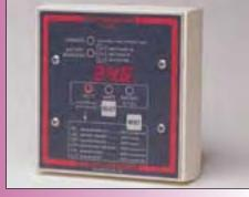
Displays vital battery system data to help users provide better battery care, increase conservation awareness and aid system maintenance. • Volts • Amps • Amp-hours • Min/Max volts
