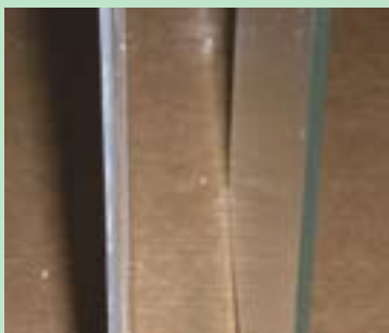
Edges of low-iron glass (clear) and window glass (green).
