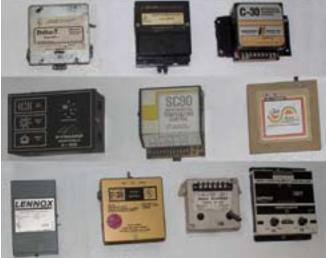
Ten differential controls used in solar water heating systems over the last 20 years.
