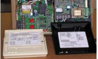
A Goldline GL-30 on the left and Heliotrope Delta-T on the right with the covers off. Note the diagrams and explanations on the covers.
