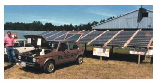
An electric "Voltsrabbit" in front of the 3 KW solar-electric array needed to provide it with a 25-mile average daily range.
