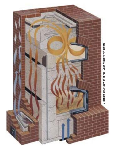
Serpentine air flow through a typical masonry stove helps warm the large thermal mass for efficient and comfortable heat.
