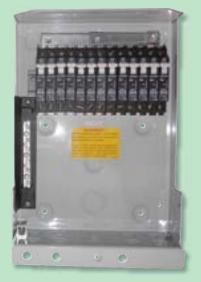
The OutBack Power Systems PSPV combiner box (shown with its cover removed) can support as many as twelve series strings of PV modules and can feed up to two charge controllers.
