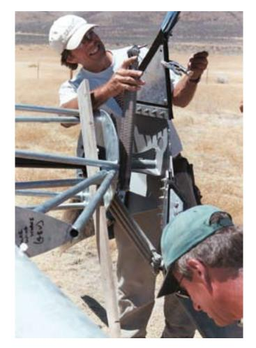
Chris attaches a spring pack, which tensions the blade, allowing it to bend back for high-wind governing.
