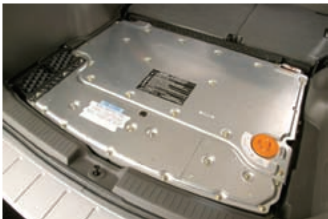
The 330-volt, nickel-metal-hydride battery stores energy for low-speed driving, and additional top-end power.
