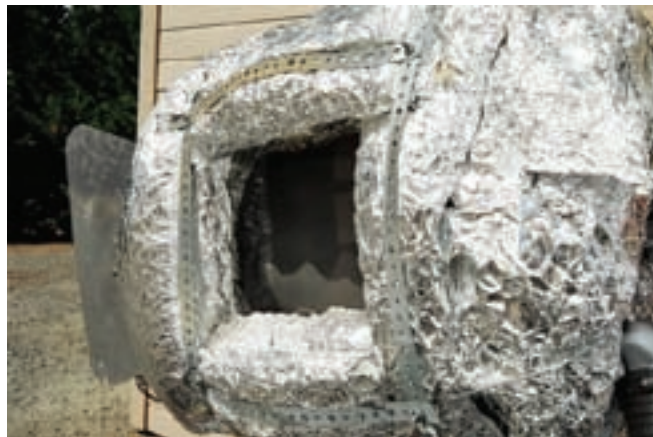
The focusing window, where all the light is aimed, heats the surface of the roasting drum inside to more than 1,200°F.
