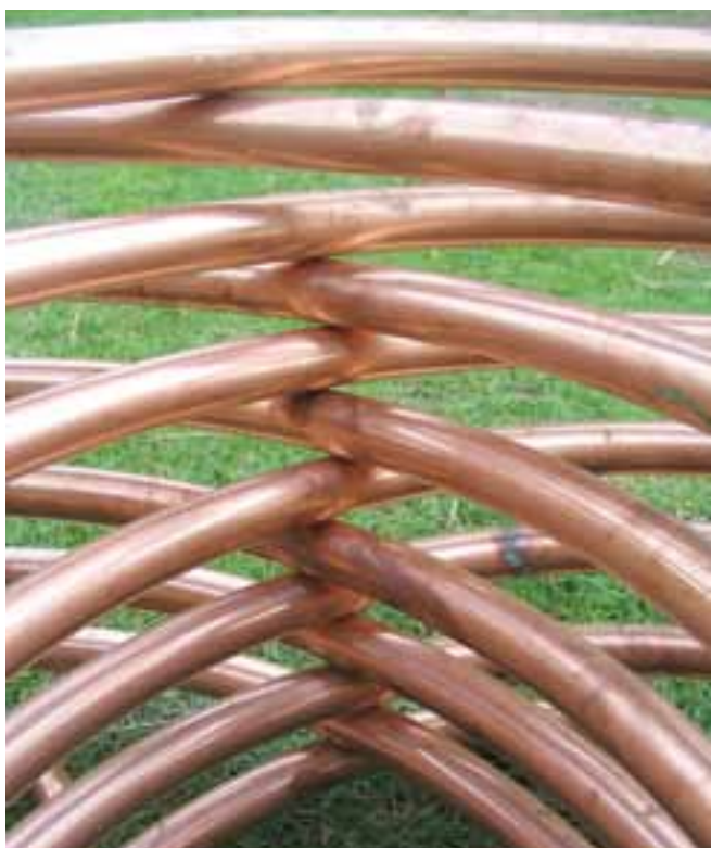
Intermingling adjacent coils saved space, separated the coils for efficient heat transfer, and allowed most of the preassembled heat exchanger to fit through the small hatch in the spring tank.
