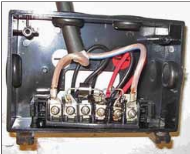
A burned diode in the junction box of a PV module, after the module was incorrectly connected to a battery.
