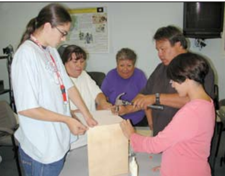
Fastening the oven box sides to the box bottom.
