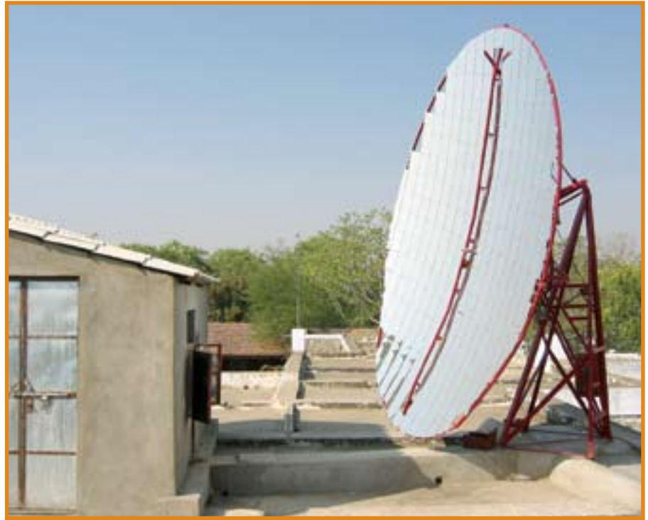
A Scheffler concentrator focuses the sun's energy into a cooking pot at Barefoot College in Tilonia, Rajasthan.
