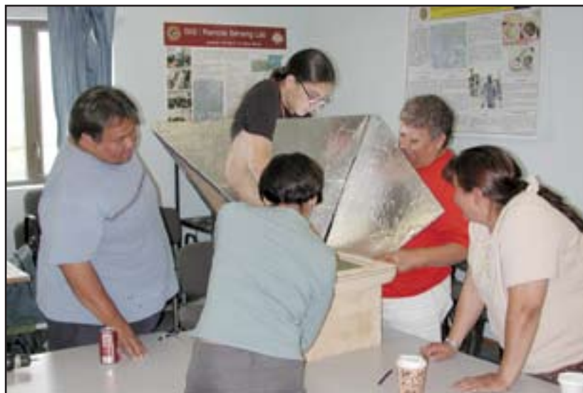
Attaching the reflectors to the top of the glass frame.
