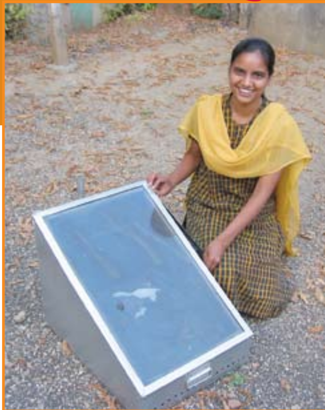
Rama Singh demonstrates a compact solar drier at the Agriculture Tools Research Center in Gujarat.
