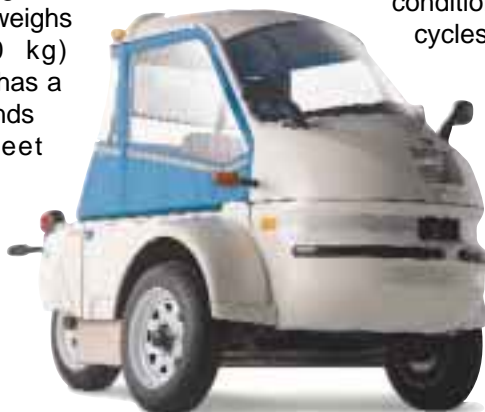
With a top speed of 40 mph (64 kph), the Gizmo is appropriate for in-town driving rather than freeways.
