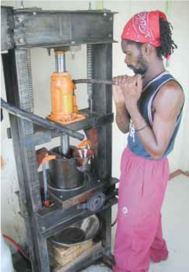
Edmond Brown works the cocoa butter press. A 24 volt homemade blender (not shown) blends up hot, ground liquid cocoa to feed the press.
