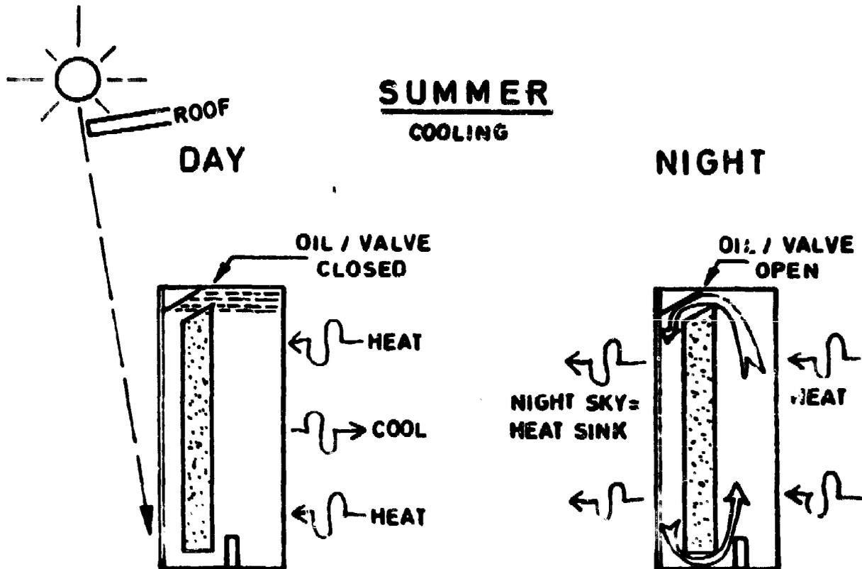
place during the day but is allowed during the night. Then the warmer water convects from the main compartment over the insulation, radiates the heat to the night environment and returns cooled below the insulation to the main compartment. The cooled water then acts as a heat sink for the building during the day.
