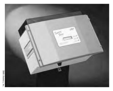
Fig. 7-3: Inverter. This quiet, efficient inverter by Sunny Boy converts direct current produced by PVs (or a wind generator) into alternating current and boosts the voltage to 120. Inverters that are used in systems with batteries typically contain battery chargers.
