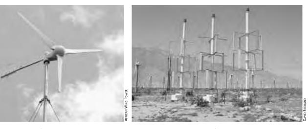
Fig. 8-4: Two types of wind machine are in use today: the horizontal axis machine shown on the left, and the much less common vertical axis machine on the right.
