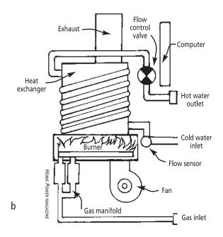
Fig. 3-2: (a) Tankless water heaters like this one heat water instantly (there's no need to store hot water for intermittent uses) and thus reduce the amount of energy required to supply a family with hot water by about 20 percent. These units are typically mounted on walls in a central location in the house. (b) Cutaway of a tankless water heater.
