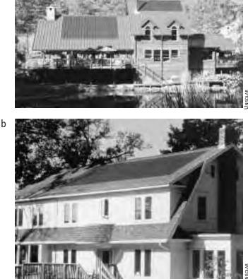
Fig. 7-12: Solar Roofing. Amorphous silicon ribbons can be used to make (a) long rolls of material that can be applied to standing seam metal roofing and (b) solar shingles. Both are forms of building-integrated photovoltaics.
