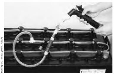
Fig. 7-9: Battery Filling System. This product is designed for those who don't want to have to top off their batteries every three or four months. Float valves in the caps tell when a cell needs replenishment. Distilled water flows into the cells from a central reservoir (not shown here).
