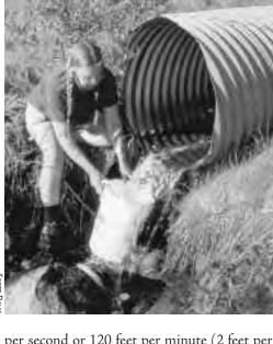
Fig. 9-6: The container fill method is one way to determine flow rates in small streams.
