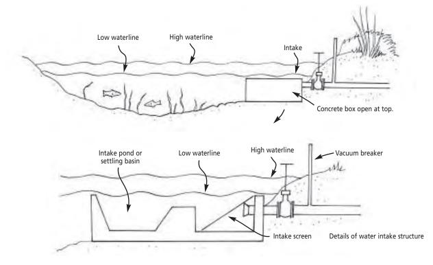
Fig. 9-4: A typical water intake structure requires a stilling basin to allow sediment to precipitate out. It also requires a deep pool so that the pipe remains free from ice. The problem with this approach is that very few people really know how long they run the TV or the toaster or the microwave each day. So estimates can be pretty inaccurate.
