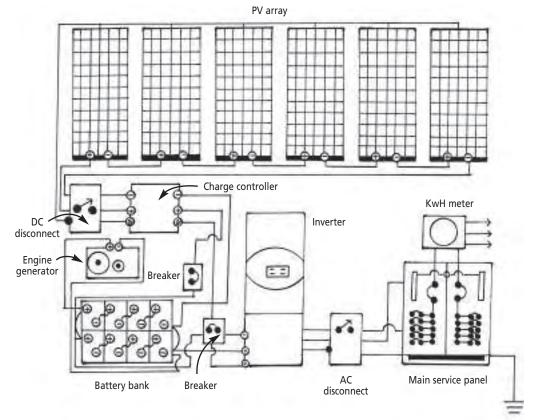
Fig. 7-6: This schematic shows all the components of a stand-alone solar electric system including charge controllers and disconnects. to enable you or a repairman to service your system without being electrocuted.
