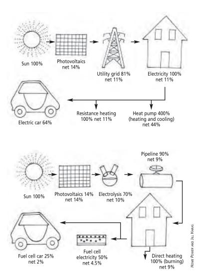
Fig. 10-2: Studying the net energy efficiency of a fuel is vital to making sound choices. This diagram from Dominic Crea's article in *Home Power* magazine, Issue 101, compares hydrogen to electricity generated from solar electricity and presents some startling findings.
