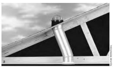
shown in Figure 4-8. Solar tube skylights consist of a small lens mounted on the roof that collects sun and directs it into a polished aluminum tube that extends from the roof to the ceiling. (The polished aluminum ensures maximum light transmission.) Light enters the room through a ceiling fixture, a diffuser that disperses light.
