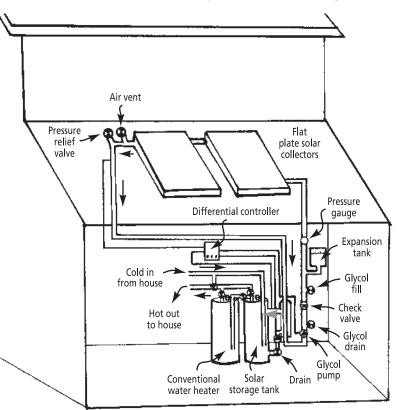
Fig. 3-11: This system uses a small electric pump to propel antifreeze (food grade propylene glycol) through a closed loop. Heat from the antifreeze solution is released at the heat exchanger, warming water in the solar hot water tank.
