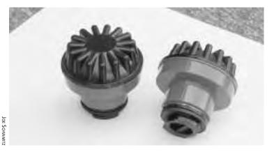
Fig. 7-8: Hydrocaps. These battery caps replace standard caps that come with lead acid batteries. The catalyst in the reservoir captures hydrogen and oxygen given off by the breakdown of water and recombines them, reducing water loss by 90 percent, thus cutting down on routine maintenance.
