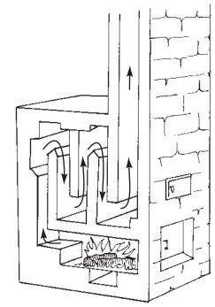
Fig. 5-11: The superefficient masonry heater relies on three features: a wellinsulated combustion chamber, a labyrinth flue, and high mass.
