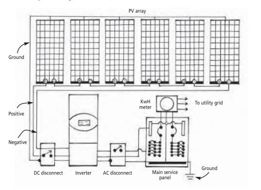
Fig. 7-4: This schematic shows all of the components of a grid-connected solar electric system, including charge controllers and disconnects.
