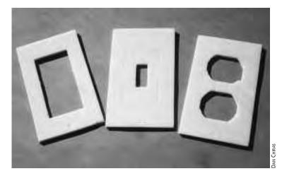
Wall switches and electrical outlets are sealed by installing small foam gaskets available in local hardware stores and larger building outlets (Figure 2-6). To seal a switch or electrical outlet, even on inside walls, remove the cover plate, then insert the foam gasket and screw the cover plate back in place.
