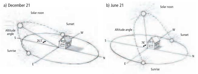
Fig. 4-1: In a passive solar home, the low-angled winter sun penetrates south-facing windows to heat the home. During the summer, the high-angled sun shines on the roofs of houses, reducing heat gain.
