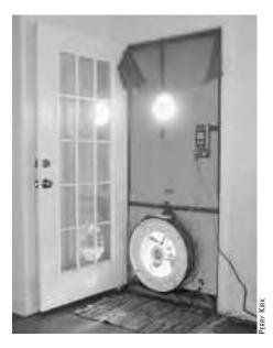
Fig. 2-4: A blower door test device like this one allows home energy auditors to determine how leaky a house is and to pinpoint the actual leaks so they can be sealed.
