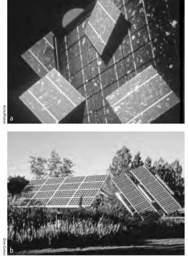
Fig. 1-5: These solar cells (a) are made of silicon dioxide which comes from sand. Solar cells convert solar energy into electricity. Many solar cells are wired together in a module which is mounted on the roof or on a free-standing rack or pole (b).
