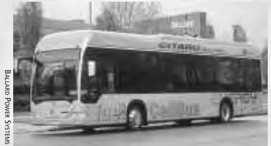
Fig. 10-4: This bus is powered by an electric motor. Electricity is generated by a Ballard Power Systems' fuel cell that is powered by hydrogen.
