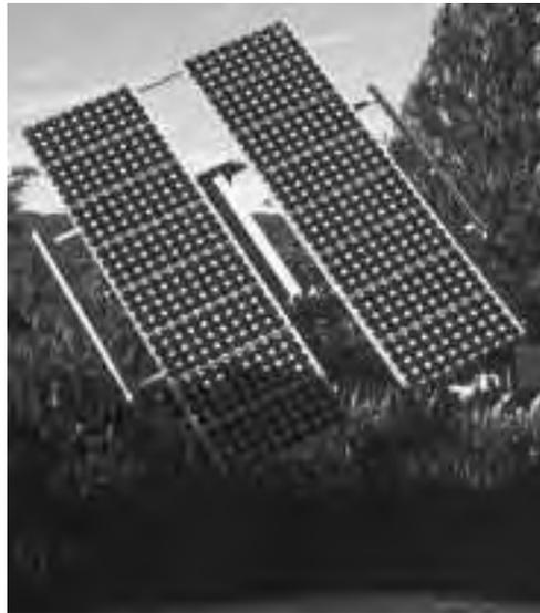
Fig. 2: These solar electric panels generate electricity from sunlight and are on a special tracking device that allows the array to move as the sun cuts its daily path through the sky. Tracking increases the efficiency of the panels by keeping the solar cells in line with the sun from sunrise to sunset.
