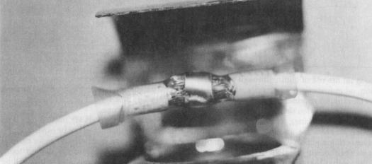
Figure 3-47. Low-temperature solder connection with built-in heat shrink tubina. The solder sleeve is just beginning to melt into the lay of the two cables. At the same time the heat shrink sleeve is starting to clamp down around the cables
