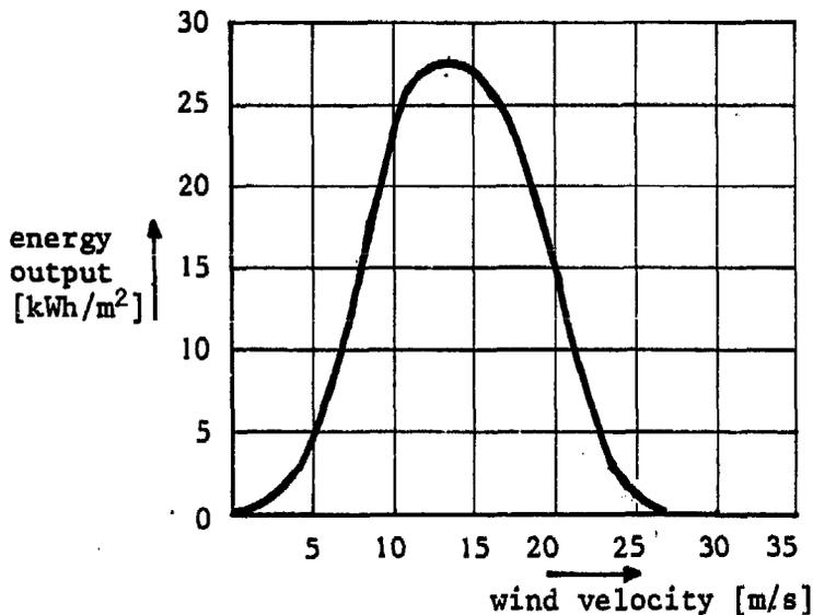
Fig. 3.7. The energy frequency curve of St. Ann's Head (U.K.), derived from fig. 3.6. with  $P = 0.1 V^3$  [W/m<sup>2</sup>]
