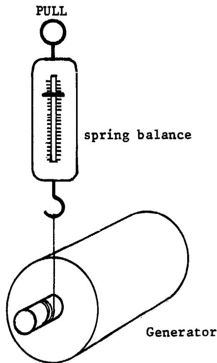
Fig. 4.26. A simple method to measure the starting torque of a generator: by gently pulling the spring balance. A force  $F$  kg can be read.
