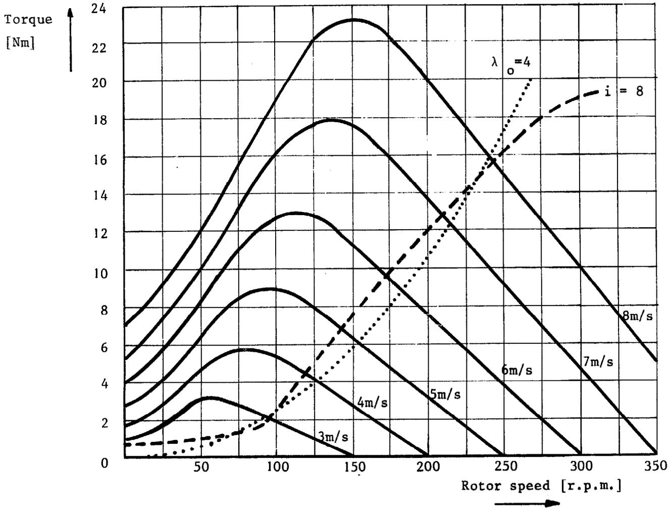
Fig. 4.27. The final torque speed curves of the wind rotor matched with a generator at transmission ratio 1 : 8, as calculated in example 4.3.4.
