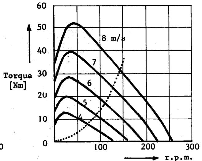
Fig. 4.2. The corresponding torque-speed curves of the rotor in fig. 4.1. for the given wind speeds
