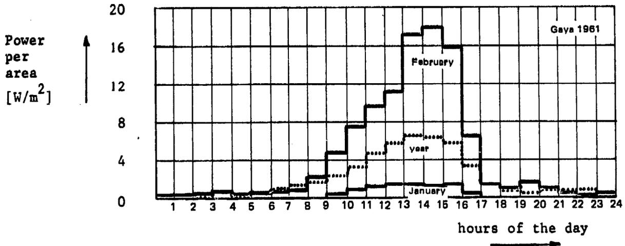
Fig. 3.5. The power distribution curve, derived from fig. 3.4, with  $P = 0.1 V^3$  [W/m<sup>2</sup>]
