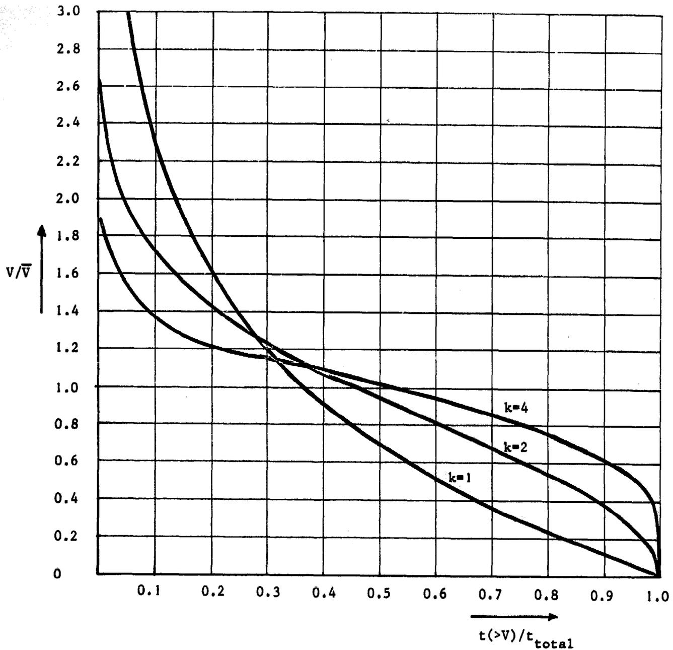
Fig. 3.9. Weibull functions, approximating (dimensionless) velocity duration curves for different wind regimes:
