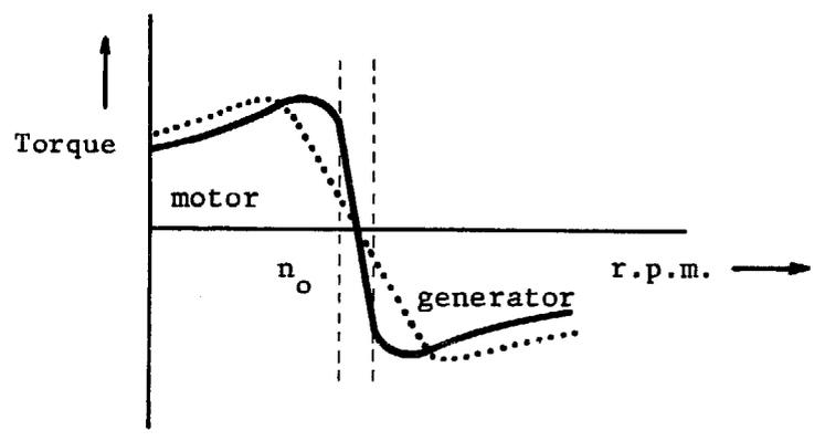
Fig. 4.10. The torque speed curve of an asynchronous machine coupled to a strong grid. Its operating range lies between  $n_0 + 4\%$  and  $n_0 - 4\%$ . The dotted curve indicates a machine with a resistance in the rotor circuit.
