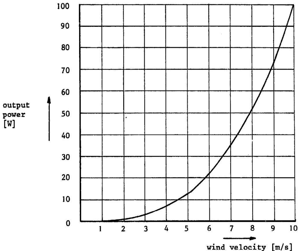
Fig. 3.2. A conservative estimate of the power output from each square metre of area swept by a windrotor:  $P = 0.1 \times V^3$  [W/m<sup>2</sup>]
