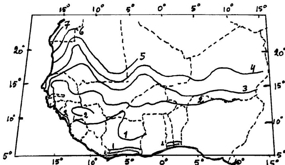
Fig. 3.3. Isovents in the Sahel area, connecting places with the same annual mean wind speed, given in m/s. The wind speeds are measured at 06, 12, 18 hours during the years 1951 to 1955 [4]
