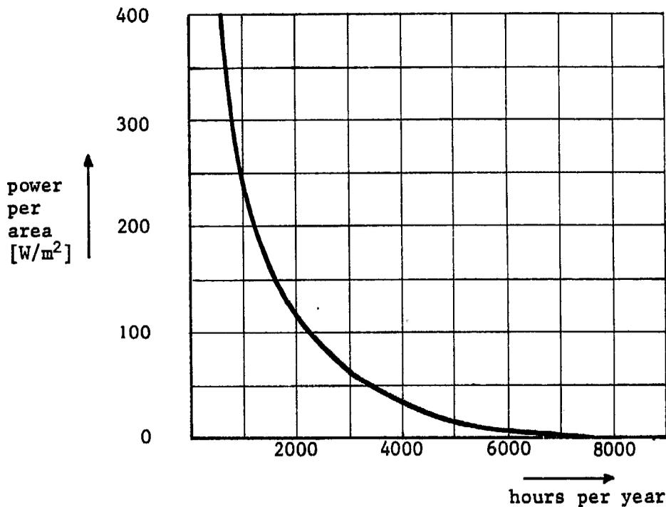
Fig. 3.10. The power duration curve of St. Ann's Head (U.K.), derived from fig. 3.8. with  $P = 0.1 V^3$  [W/m<sup>2</sup>]
