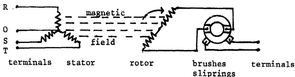
Fig. 4.7. Schematic representation of a three-phase synchronous machine
