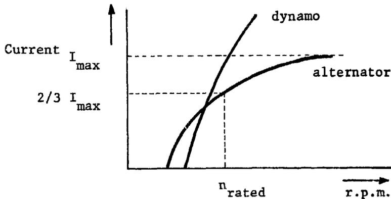
Fig. 4.12. The output current  $I$  as a function of the rotational speed of a dynamo and an alternator
