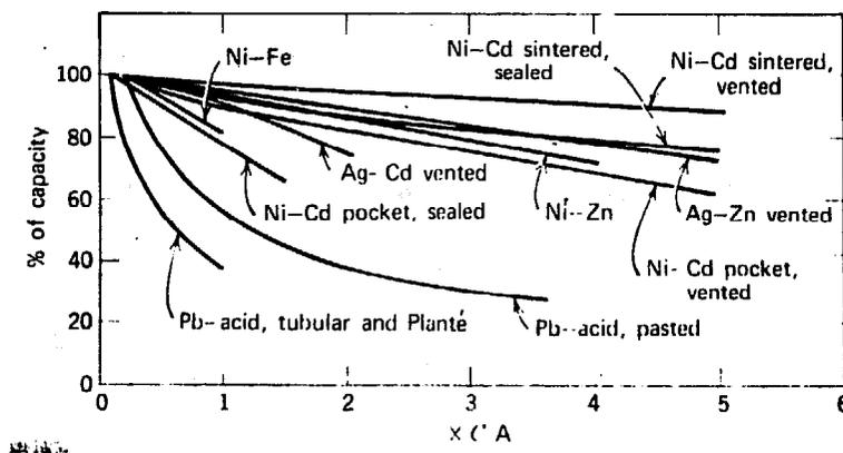
Fig. 5.2. The capacity of different electrolytic cells as a function of multiples of the nominal discharge current.
