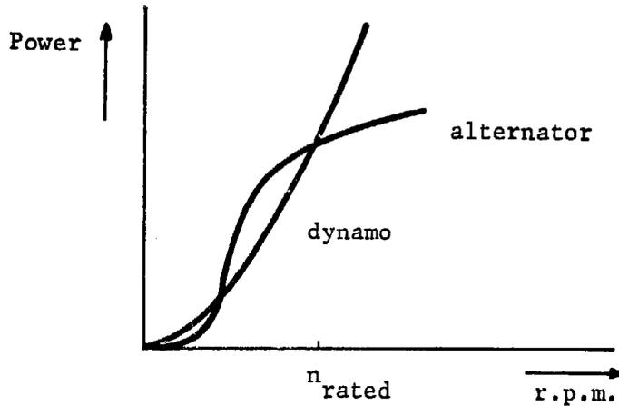
Fig. 4.14. The power output curves of a dynamo and an alternator
