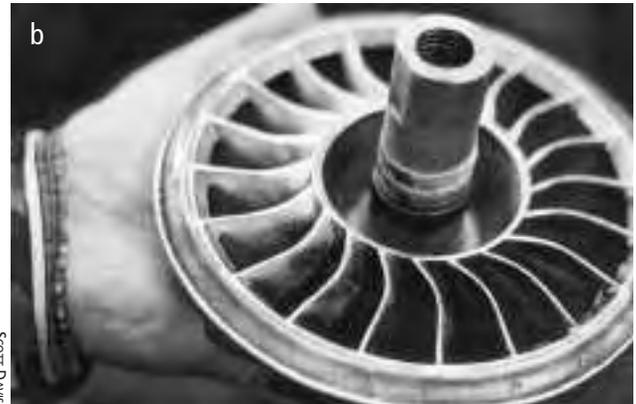
Fig. 9-3: (a) Pelton and (b) Turgo turbines.
