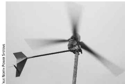
to rotate the machine around the yaw axis. However, the tail resists this rotation and keeps the rotor facing into the wind.
