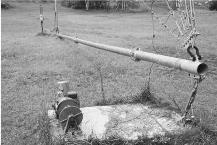
Fig. 6.12: *Gin Pole. The gin pole is attached to the anchor. Notice the electric winch to the left of the attachment.*
