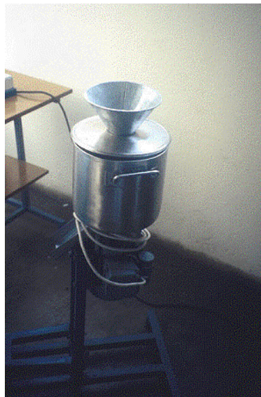
ITDG Southern Africa Example of equipment sold in the light engineering workshop - Peanut Grinding Machine.
