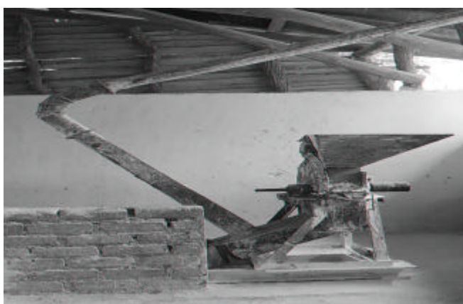
Figure 1: Swing hammer mill being used for lime milling in Malawi. ITDG.
