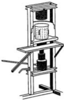
speed up removal of oil. The pressure should be increased slowly to allow time for the oil to escape. Screw types are more reliable than hydraulic types but are slower and produce less pressure. Except where a lorry jack is used (Figure 4), hydraulic types are more expensive, need more maintenance, and risk contaminating oil with poisonous hydraulic fluid.
