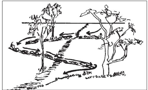
Figure 4.2 Redirected water flow is slower and more beneficial after swales or contouring.
