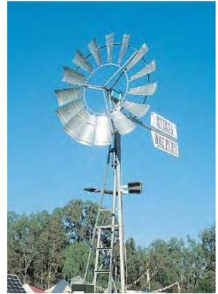
Windmills provide a clean and cheap way of pumping water on the farm.
