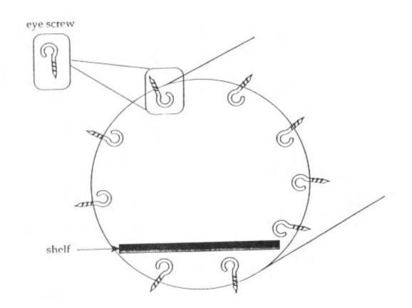
Corrugated roofing metal or other types of sheet metal are ideal materials for blocking culverts under roads. Use your ingenuity to affix them to the cul-vert so they will stay in place in high water. (Try using eye bolts as suggested above, or drive large nails into the walls of the culvert.)
