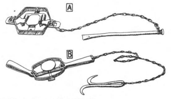
A) Coil spring-type trap attached to stake.
