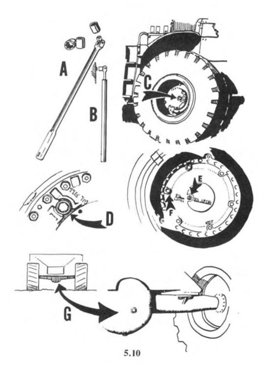
Various types of oil filler caps found on wheel hubs can be seen in (C) through (F). In (G) is a plug in a differential through which lubricating oil (and abrasives) is introduced. A neat job will ensure that even if the operator checks, abrasives will not be immediately apparent.
