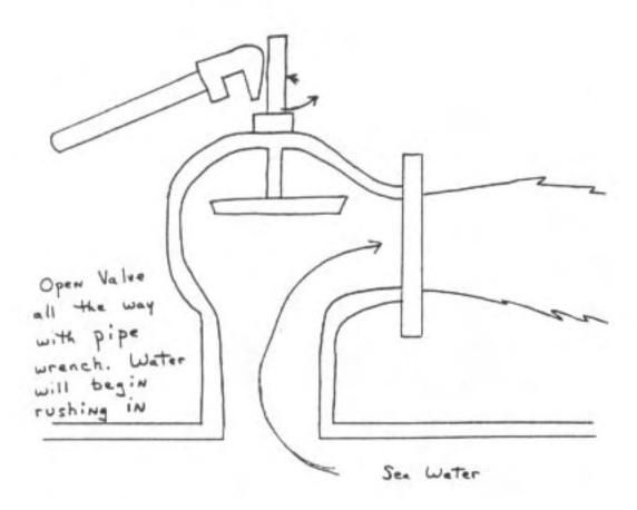
With your wrench, bash and bend the valve stem so that it will not be possible to close the valve.
