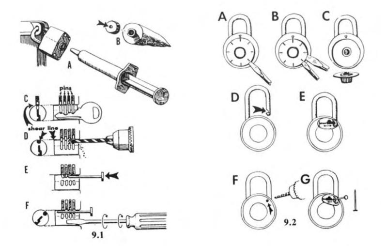
Inserting a pin, like a nail, will keep the damaged remains of the top pins above the shear line. Otherwise they will drop down and prevent the lock from opening. You may need to put the drill bit in a couple of times to chew up any pin fragments that might interfere with opening. Finally, insert a narrow-bladed screwdriver (F) into the keyway and turn it to open the lock. Before using this method in the field, buy a cheap padlock or two and practice at home.
