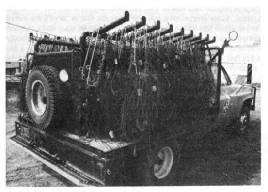
Truck with seismic cable.
