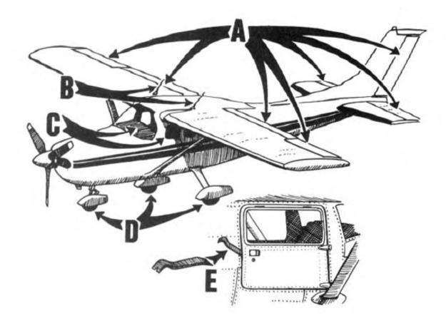
E. Instruments. Use a regular prybar from a hardware store to force open the door of an airplane. Once inside, use the end of the prybar to demolish the instrument panel.
