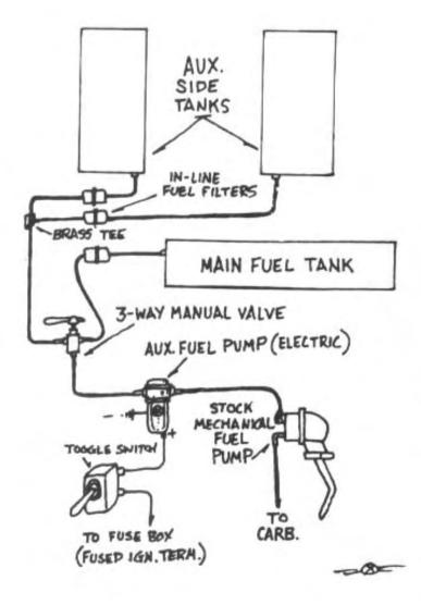
NOTE: MOUNT ELECTRIC PUMP ON FRAME TO AVOID EXCESSIVE NOISE AND VIBRATION HAVE PARTS TO BY-FLSS MECHANICAL PUMP ON HAND (IN CASE OF LEAKS)
