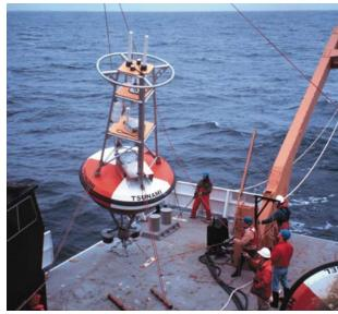
Tsunami buoy being deployed in the Pacific Ocean. Source: NOAA
