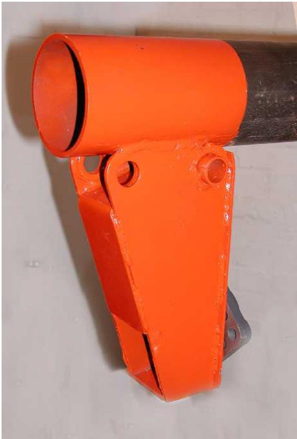
This first "tailstock" was made from an old piece of service station jack that had a 7/8" flange bearing added. For alignment purposes, it was step drilled with bits held in the lathe chuck. It has worked very well for the last three years.
