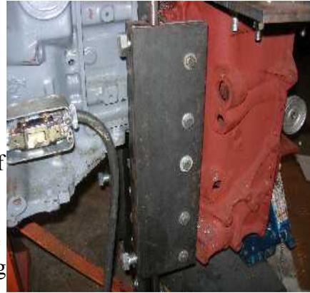
(2) **The drive unit module.** There are literally dozens of ways to drive the machine. A combination of small and large pulleys makes a good medium-speed drive. Other setups might include multiple-groove pulleys or even the transmission from a lawn mower, garden cultivator, or pickup truck. Power can be provided by anything from an electrical appliance motor to a car or truck engine.
