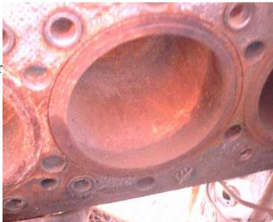
These cylinders can have aluminum alloy liners cast into them and then machined to the right size with the temporary lathe. Sounds like a big job? Sure, but you can make a machine can have the capacity of a machine tool that would cost over a hundred thousand dollars in the USA and several times that elsewhere.
