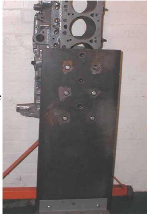
You may also use the #1 cylinder for the spindle if you don't need your machine to be a horizontal mill that would normally use this cylinder for the overarm. eBay makes horizontal mills extremely useful because of the cutters often being available at 95% discount. Even if you don't have access to cheap cutters, a homemade fly cutter is much easier to make than a homemade end mill.
