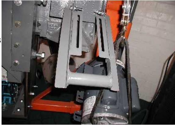
Again, it would be best if the pulleys were mounted inboard the mounting rails if possible. Be sure to lay everything out first so you can be sure the motor and pulley assemblies all fit properly. Work carefully here and you will get a quiet, powerful machine that is less likely to "chatter".
