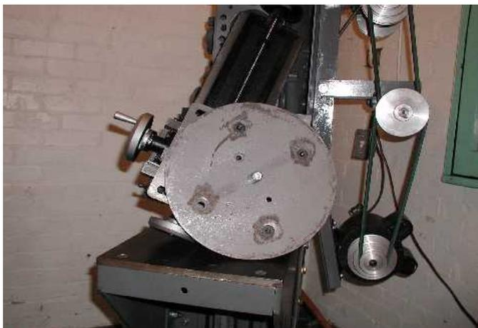
If you use a "store bought" cross slide then mount it on a turntable. The turntable can serve as a lathe compound. If you make the turntable 11.46 inches in diameter then a 36" length of 1/4" tape measure will give you 360 degree graduations at one and a quarter degrees each! **Be sure to check for clearance for bottom cross feed knob. You may have to add a spacer for clearance.**
