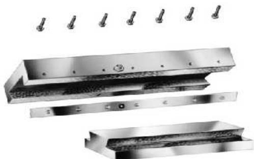
Long, angled cuts similar to this commercial dovetail assembly on the cross slide shown below would be far more difficult to build than the MultiMachine's simple, square sections that are bolted together. **While the MultiMachine vertical slide requires only a drill to build, a long dovetail requires a very large milling machine. A hugely important difference!**
