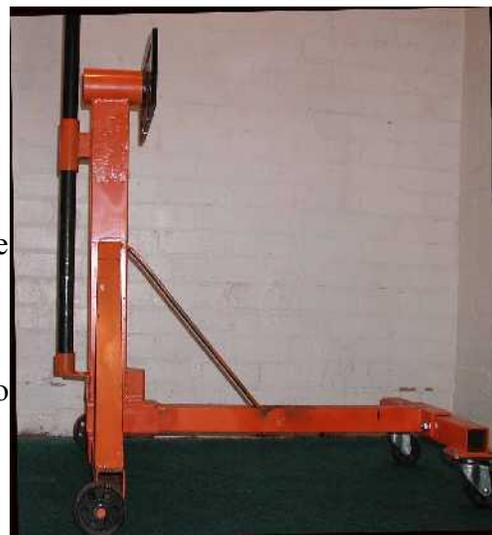
(4) **The overarm module** may not even be needed by some people but others may see it as the heart of an entire tooling system. Because it is important that the overarm always stay in alignment, *the #1 cylinder is re-bored to fit your overarm pipe at the same time the #3 cylinder is re-bored for the spindle.*
