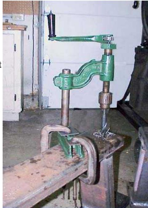
This particular drill was a ratchet drill made by the Cole Tool Company. The power of this type of tool lies in the feed screw that can be tightened down by hand, exerting extreme pressure on the drill point. Materials such as spring, stainless and tool steel can be drilled with by using ordinary high speed steel or masonry carbide type drill bits. The Cole Drill is still useful for drilling large holes in hardened steel or workpieces that are too large for the drill press.
