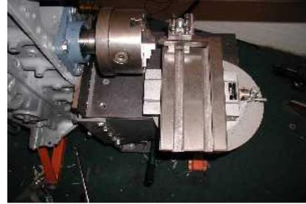
**It can face and cut tapers by simply rotating the cross feed on the "turntable."**
