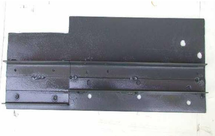
There are almost unlimited ways to power the machine but no matter how you plan to power your machine, you will probably need a mounting plate like this one that I made from scrap. It is securely bolted to the side of the block. Make it as long and wide as possible and use 1/4" plate if possible. I used 3/16" and it tended to flex under load.
