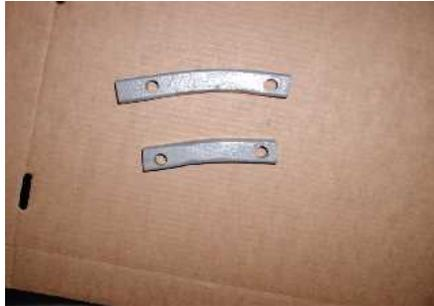
Top view of a set of clamps made from an old piece of one inch key stock.
