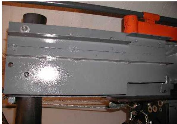
Here the plate is shown bolted to the side of the block.
