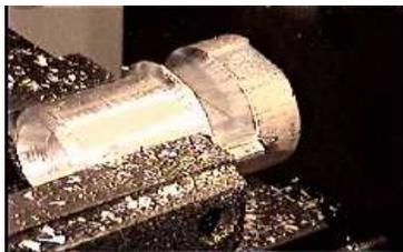
**My MultiMachine made a 400rpm single pass-cut of .822" x 1/2" in this piece of 6061 aluminum.**
