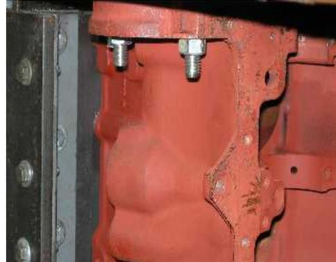
**The drawings on the next two pages show the current clamp mechanism. By properly adjusting the top and bottom 3/4" clamp bolts (putting a little more pressure on the bottom clamp bolt than on the top) and adding a little pressure with the jack, the vertical slide can be raised in increments of .0001" (by light taps!) and the table does not move when the clamp bolts are tightened!**
