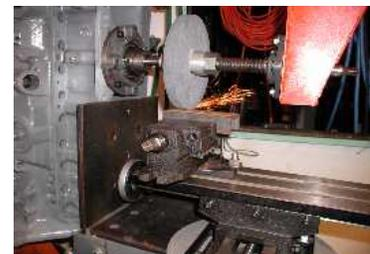
**Other arbors can be easily made for fly cutters, wood and metal saw blades, surface grinding wheels and sanding drums and discs.**
