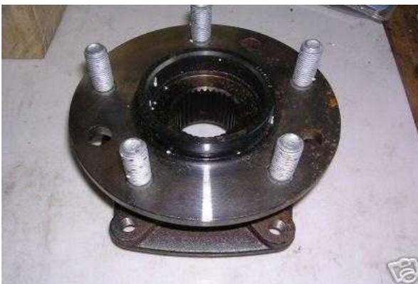
A really simple "temporary" lathe, use a hub from a front wheel drive car. The cutting tool can be as simple as a large allen wrench (good steel) ground to the proper shape and attached to a long handle. Blacksmiths used this technique on iron and steel for many years and using it on zinc/aluminum alloy will be much easier. This is another very good reason to learn the basics of tool grinding.
