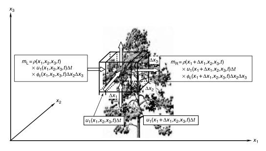
**FIGURE 14.2** Air mass flow in the Lagrangian control cube where  $m_L$  is the mass of air into the cube through the left slice over a time interval  $(\Delta t)$ ;  $m_R$ , the mass of air out of the cube through the right slice over  $\Delta t$ ;  $u_1(x_1, x_2, x_3, t)$ , air velocity in the  $x_1$  direction;  $\rho(x_1, x_2, x_3, t)$ , air density;  $\phi_C(x_1, x_2, x_3)$ , cubic porosity; and  $\Rightarrow$ , the direction of air motion.
