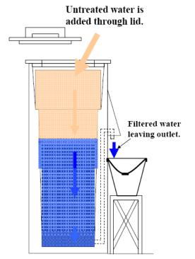
Recall that the BioSand Water Filter will remove 100% of parasites (protozoa) and larger microorganisms (helminthes).
