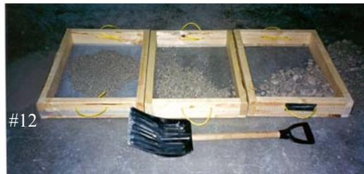
13 – 19. Process of washing the filtering media. Note that filtering media may not be washed to completely clean as was the underdrain and separating media.
