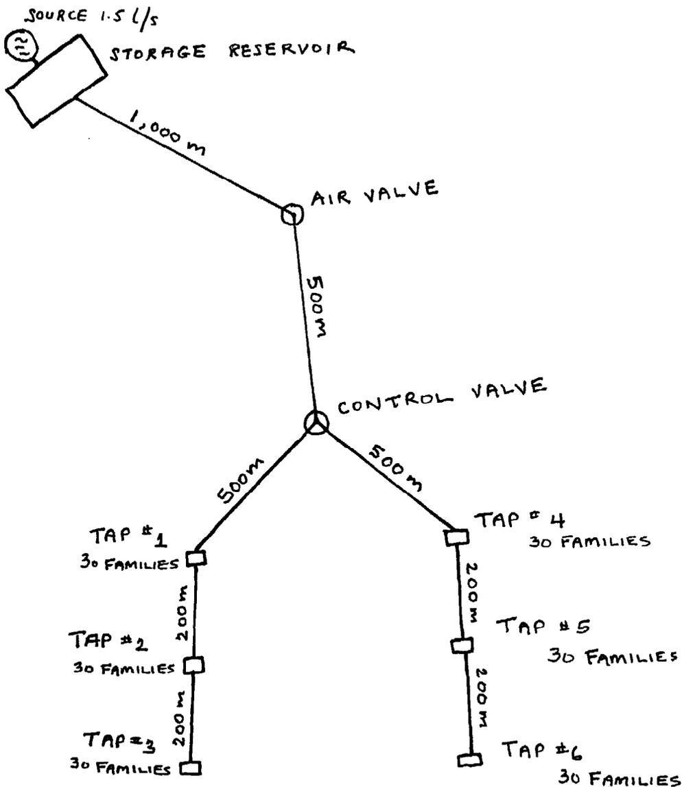
P.20.1. In this system a storage reservoir will be constructed at the spring. Recommend an appropriate volume for the reservoir? How was the volume calculated? Suggest approximate dimensions for the reservoir.
