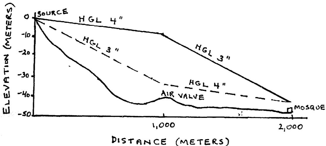
a. Both configurations will result in approximately the same amount of water flowing to the mosque. If the 3 inch pipe is placed first then there is a greater amount of turbulence and a greater head loss at the transition point between the 3 and 4 inch pipes. The flow in the transition area from a 4 inch to a 3 inch pipe is smoother and results in a smaller head loss. However, for this particular situation the effect is negligible.
