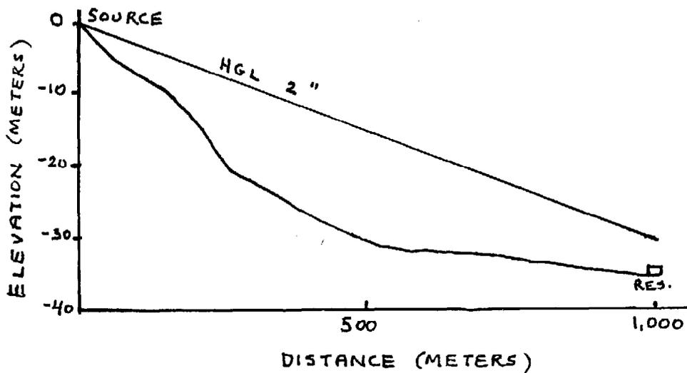
P.14. Given the ground profile and design flow in the figure below choose appropriate GI pipe. Plot the HGL for the pipe selected.
