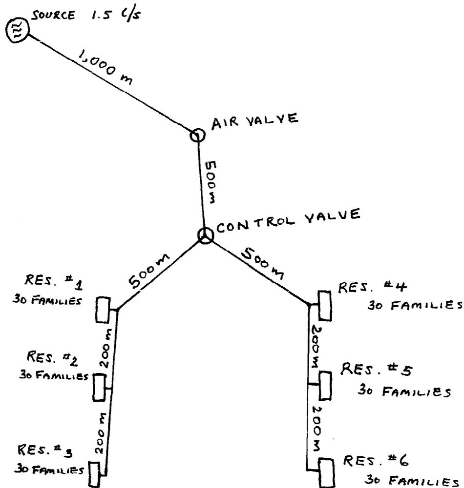
P.22.1. In this system six small reservoirs will be built in the kampong. Recommend an appropriate volume for the storage reservoir. How was this volume calculated? Suggest approximate dimension for the reservoirs.
