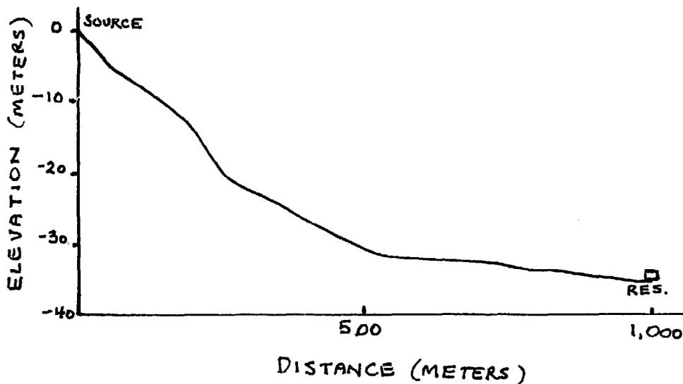
S.13. The available head from the source to the reservoir is approximately 35 meters. Using the water flow calculator the following values are obtained for a flow of 2 l/s using GI pipe :
