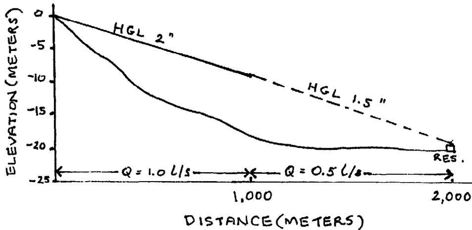
P.15. Given the ground profile in the figure below plot the HGL for a design flow of 4 l/s using 3 inch GI pipe.
