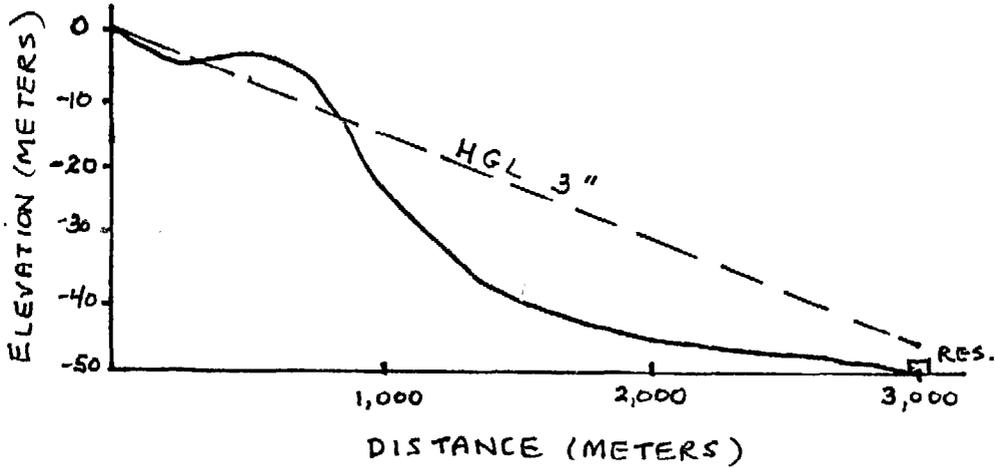
a. If the 3 inch pipe follows the ground profile then it will lie above the HGL near the source. This means that there could be a negative pressure in the pipeline in this area. Thus, three inch pipe is not suitable.
