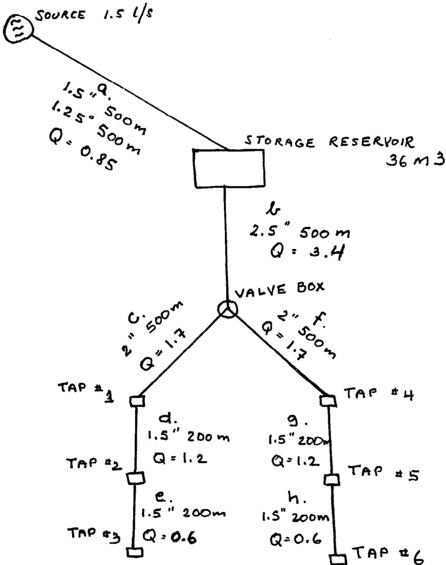
S.21.6. The manufacture of "krupuk kanji" requires the use of water and the design flows should be increased to supply the necessary amount. For example two small processing areas could be located near taps # 1 and # 4. If each area were supplied with 0.2 l/s (or 17.2 m<sup>3</sup>/day) then the design flow for sections a and b would be increased by 0.4 l/s and the design flows for sections c and f by 0.2 l/s.
