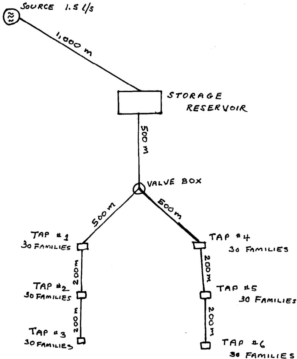
P.21.1. In this system a storage reservoir will be constructed 500 meters from the village. Recommend an appropriate volume for the storage reservoir. How was this volume calculated? Suggest approximate dimensions for the reservoir?
