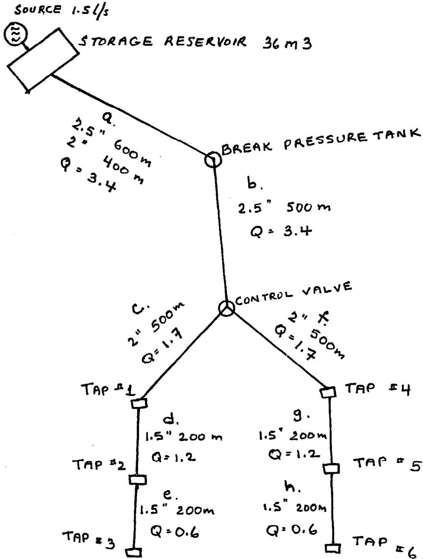
P.21. The Department of Local Transmigration is building a small kampong which will eventually have a population of 900 persons. They are planning to build a small gravity fed water system using a spring above the kampong with an estimated minimum flow of 1.5 l/s. Each person should receive at least 80 liters per day of water which will be distributed to 6 public tap areas. The figure below is a general sketch of the village and planned distribution system.
