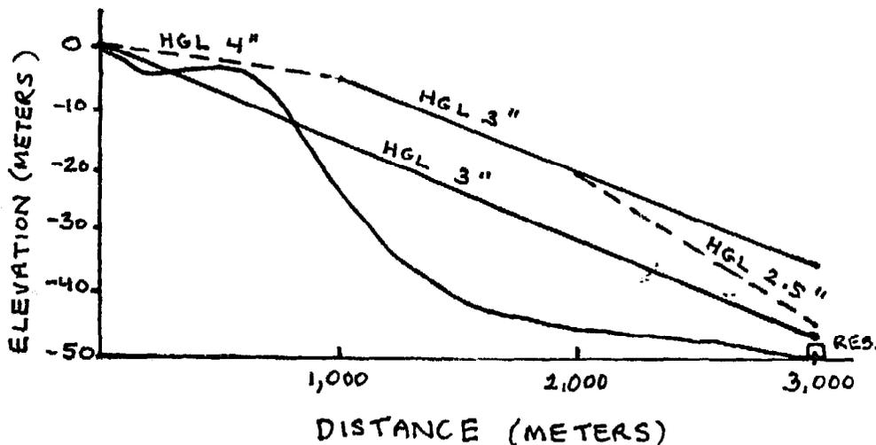
P.17. The figure below contains a ground profile from a water source to a reservoir located at a mosque 2,000 meters from the source. An air valve is located 1,000 meters from the source. The design flow for this section of pipe is 6 l/s. Plot the HGL for 4 inch pipe from the source to the air valve and 3 inch GI pipe from the air valve to the mosque. Now plot the HGL using 3 inch GI pipe from the source to the air valve and 4 inch GI from the air valve to the mosque.
