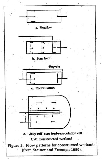
Whatever the configuration, care must be taken to ensure equal flow distribution at the inlet and to avoid short-circuiting of flow to the outlet.
