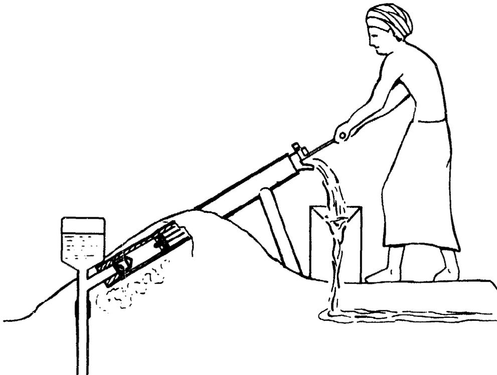
Fig. 90 Rower pump (part sectioned) (after Klassen [28])
