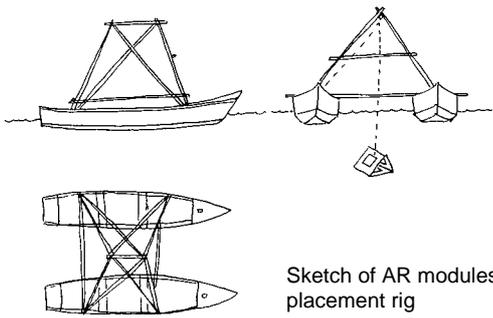
modules off the boats (in this case kattumarams) which have ferried the modules out to the rig, and lower them onto the seabed. The site for the reef is chosen by the community, and is marked out to ensure that it is oriented across the current.
